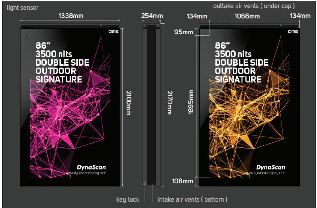
Digital Signage Panel Dimensions. NTS (Source: Dynascan)
