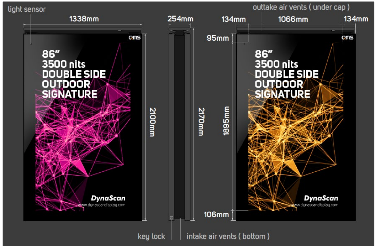
Digital Signage Panel Dimensions. NTS (Source: Dynascan)
